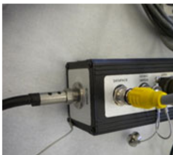
Figure 17 Cone Cable and Datapack Cable to Connector Hub ENCL-0026
